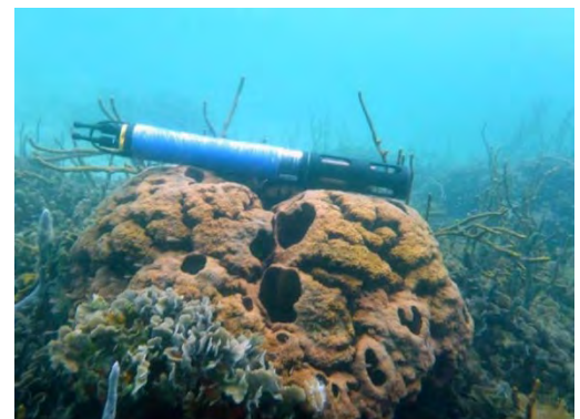
Sonde measuring water quality parameters on a coral reef.
