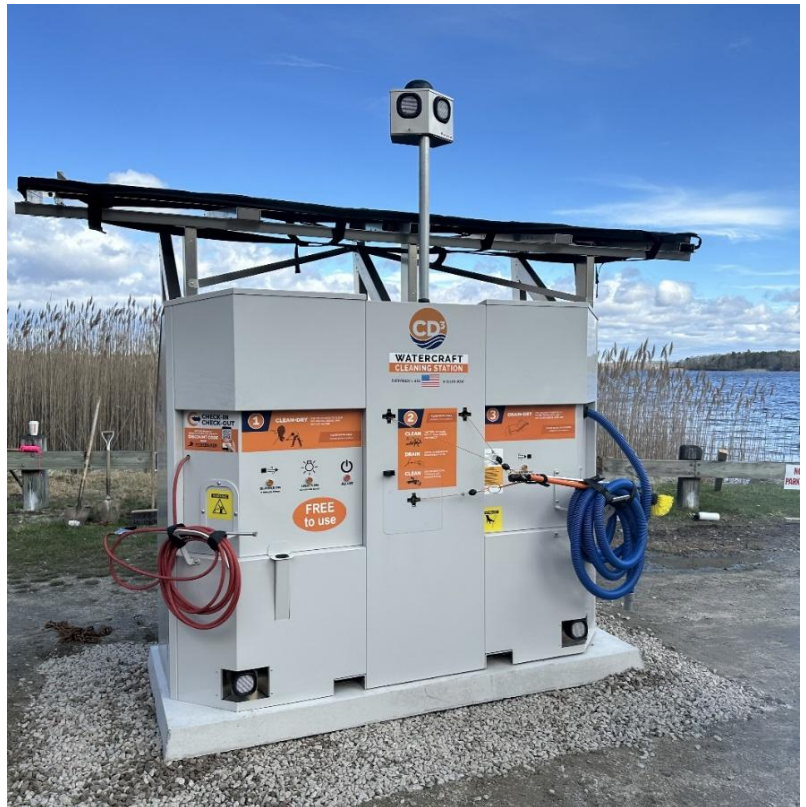
The solar-powered boat cleaning station stands to remind boaters to clean off their boats and provides compressed air to dry gear, a wet-vacuum to remove water and plants, and tethered tools available to reach difficult spaces under boat trailers.
